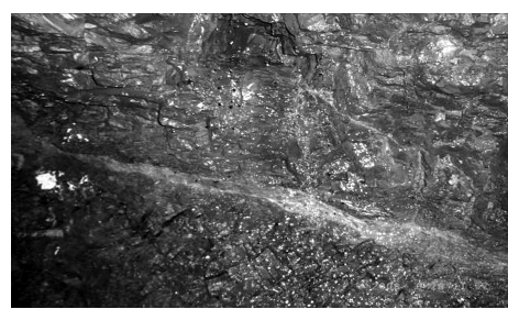
图 7 深卸荷与缓倾角错动带示意图(据文献[29]) Fig. 7 DSC and shear belt
