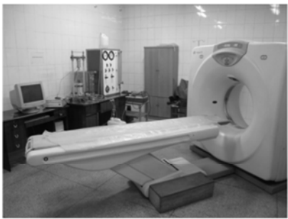
图 1 后勤工程学院 CT-三轴试验研究工作站 Fig. 1 CT-triaxial experimental research workstation of Logistic Engineering University of PLA
