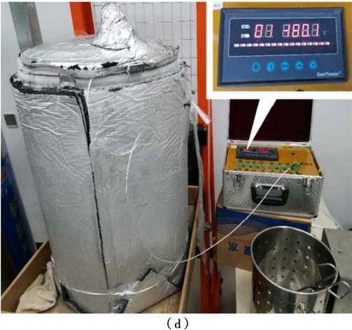
图 1 超低温冻土单轴压缩试验过程 Fig. 1 Uniaxial compression test process of ultra-low temperature frozen soil
