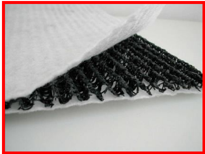
图 1 “M”型新型排水垫构件 Fig.1 Components of “M” type filter structure
